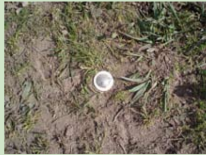
Soil erosion marker installed at outer reaches of erosion.
